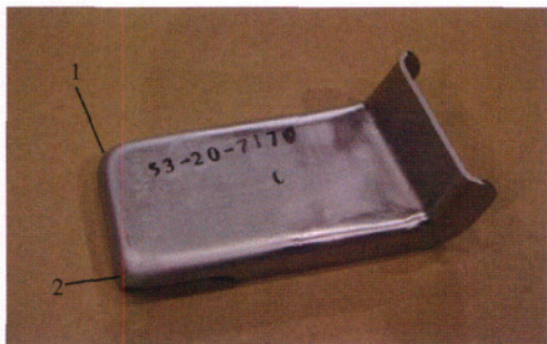
图7 中心顶出成形方案成形后的零件 Fig.7 Part after forming by using central push-out method
